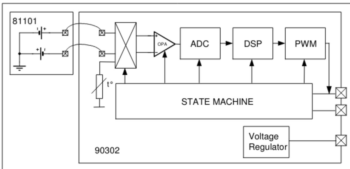
Figure 3: block diagram
