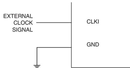
When this clock source is selected, start-up times are determined by the SUT Fuses as shown in Table 7.
