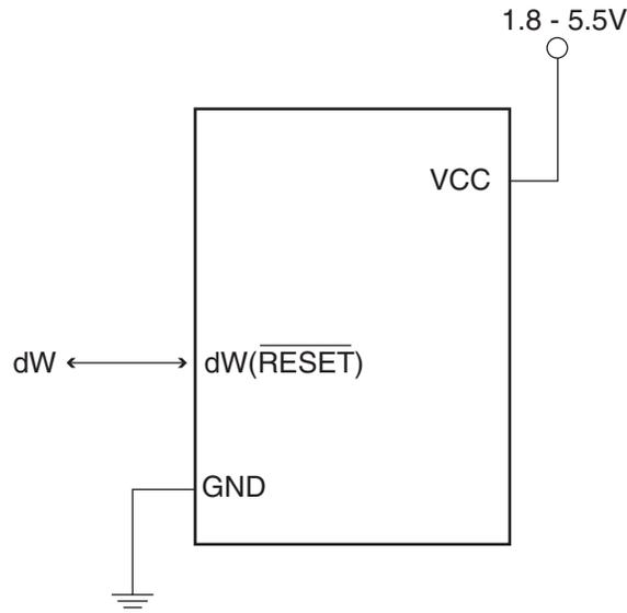
Figure 52 shows the schematic of a target MCU, with debugWIRE enabled, and the emulator connector. The system clock is not affected by debugWIRE and will always be the clock source selected by the CKSEL Fuses.
