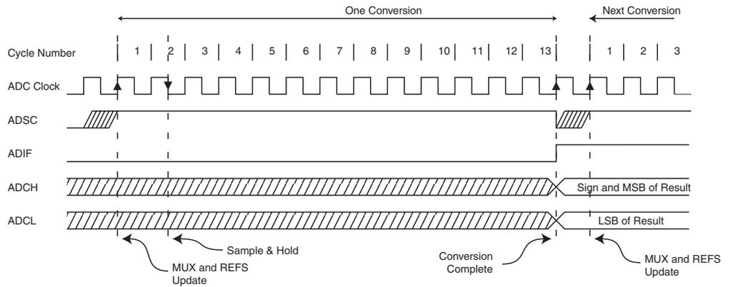
**Figure 45. ADC Timing Diagram, Auto Triggerred Conversion**
