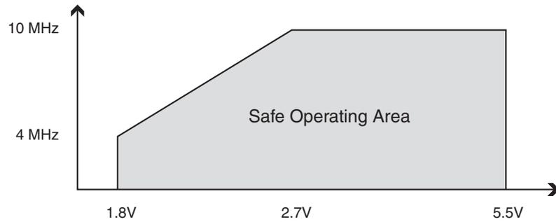
**Figure 63.** Maximum Frequency vs.  $V_{CC}$ , ATtiny13
