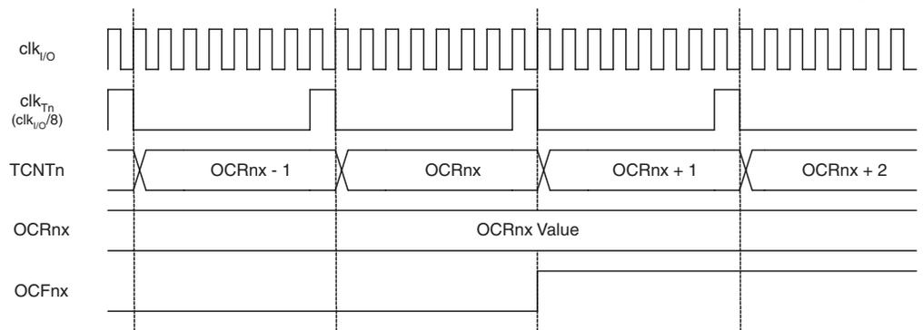
Figure 36 shows the setting of  $OCF0A$  and the clearing of  $TCNT0$  in CTC mode and fast PWM mode where  $OCR0A$  is TOP.
