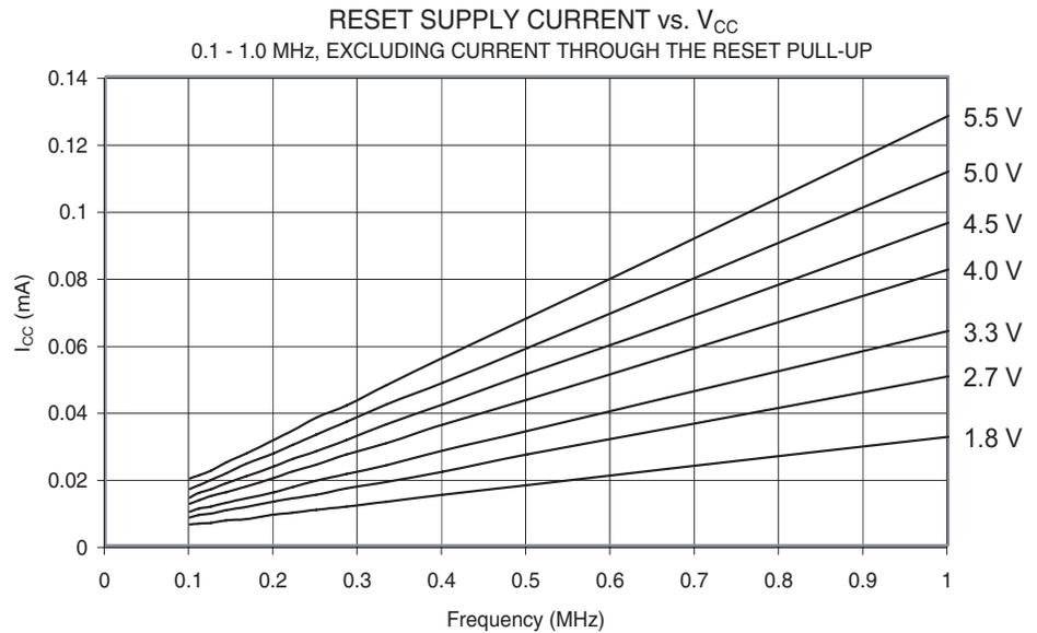
**Figure 128.** Reset Supply Current vs.  $V_{CC}$  (1 - 24 MHz, Excluding Current through the Reset Pull-up)
