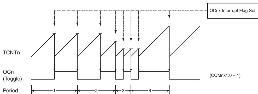
An interrupt can be generated each time the counter value reaches the TOP value by using the OCF0A Flag. If the interrupt is enabled, the interrupt handler routine can be used for updating the TOP value. However, changing TOP to a value close to BOTTOM when the counter is running with none or a low prescaler value must be done with care since the CTC mode does not have the double buffering feature. If the new value written
