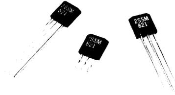
2SS52M Series position sensors have a built-in magneto-resistive bridge integrated on silicon and encapsulated in a plastic package. The integrated circuit also includes a band-gap regulator and a digital output that will respond to very low magnetic fields. Though the signal is identical to our digital Hall effect sensors, it can be achieved by magneto-resistive sensors at much greater sensor-to-magnet distances.
