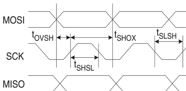
**Table 51.** Serial Programming Characteristics,  $T_A = -40^{\circ}\text{C}$  to  $85^{\circ}\text{C}$ ,  $V_{CC} = 1.8 - 5.5\text{V}$  (Unless Otherwise Noted)
