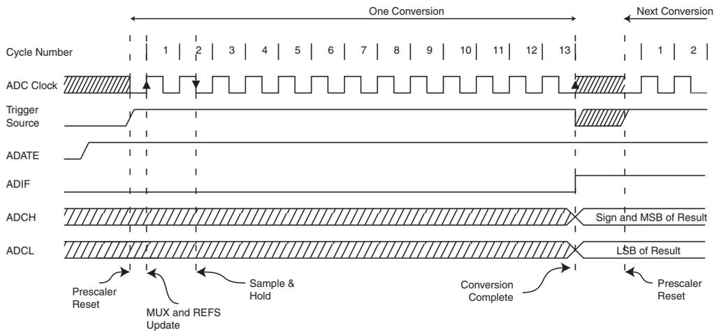
**Figure 46.** ADC Timing Diagram, Free Running Conversion
