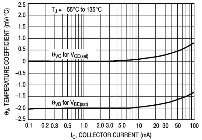
Figure 5. Temperature Coefficients
