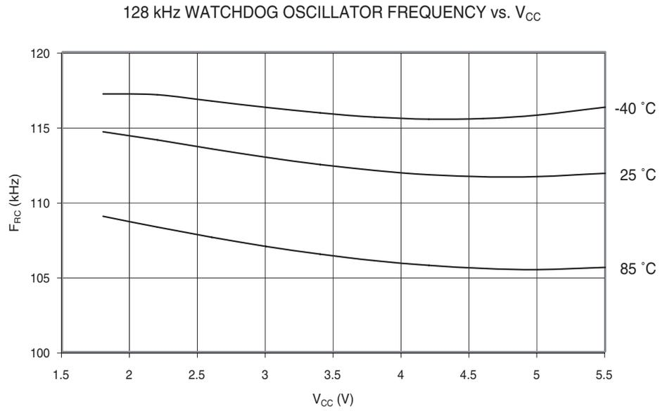
**Figure 122.** 128 kHz Watchdog Oscillator Frequency vs. Temperature
