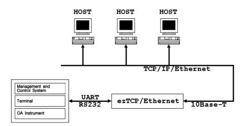
If a host computer (hereafter a host) is connected to the TCP port of ezTCP over an Ethernet network, the serial port of the DTE is connected virtually to the TCP port of the host. Then, ezTCP will function as an intermediate device between the serial port and the TCP port.
