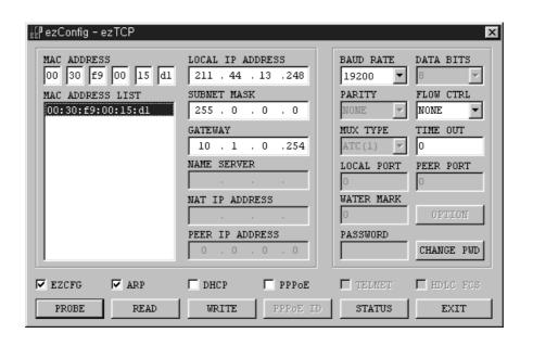
On ezConfig, set [LOCAL IP ADDRESS], [LOCAL PORT], and the serial port setting to be consistent with the test environment. After completing the setup, press [WRITE] button to save the changed values in ezTCP. If an error message appears during storing the setting, check if ezTCP is connected correctly, and then try again.
