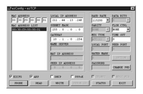
Run HotFlash to enter IP address in the IP address window according to ezConfig. The following picture shows the IP address, which is set to 211.44.13.248:
