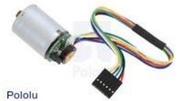
Key specs at 6 V: 5600 RPM and 80 mA free-run, 1 oz-in (0.07 kg-cm) and 2.2 A stall.
