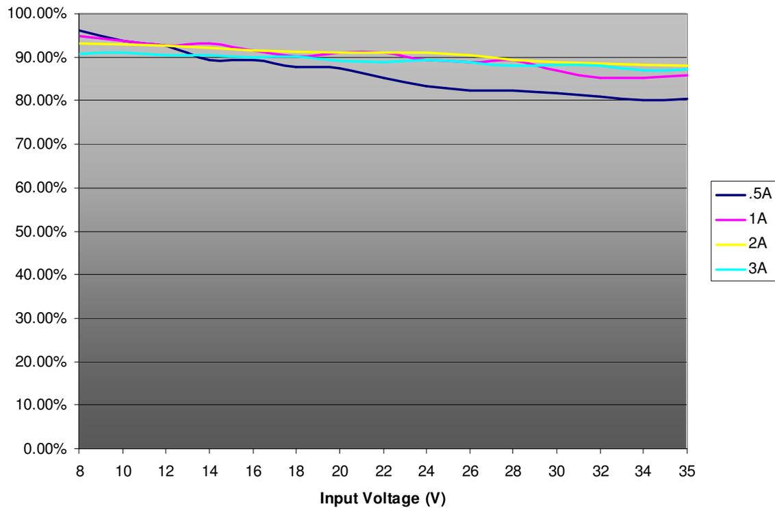
**Efficiency % vs. Input Voltage at 3 Volts Output**
