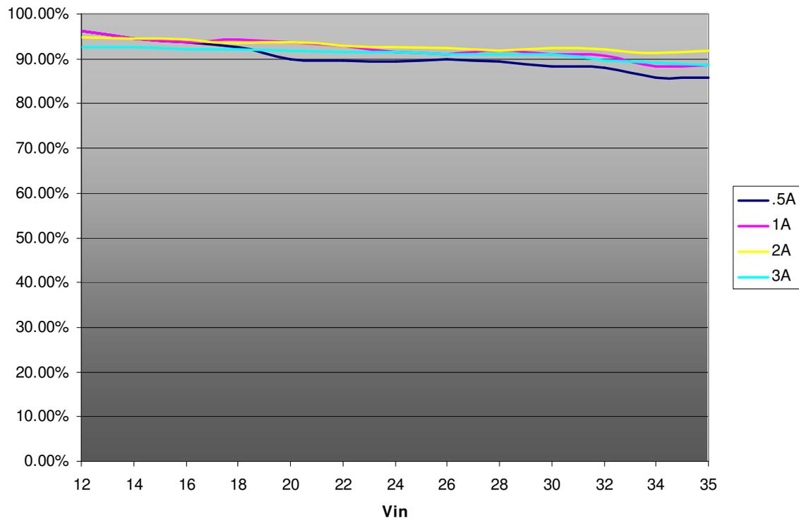
**Efficiency % vs. Input Voltage at 6 Volts Output**
