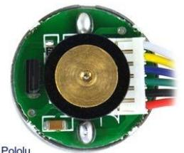
The Hall sensor requires an input voltage,  $V_{cc}$ , between 3.5 and 20 V and draws a maximum of 10 mA. The A and B outputs are square waves from 0 V to  $V_{cc}$  approximately 90° out of phase. The frequency of the transitions tells you the speed of the motor, and the order of the transitions tells you the direction. The following oscilloscope capture shows the A and B (yellow and white) encoder outputs using a motor voltage of 6 V and a Hall sensor  $V_{cc}$  of 5 V:
