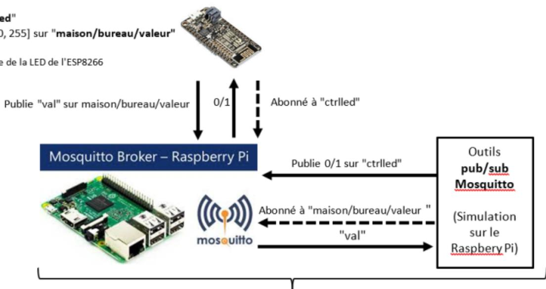
**Raspberry Pi - Simulation Client MQTT**
